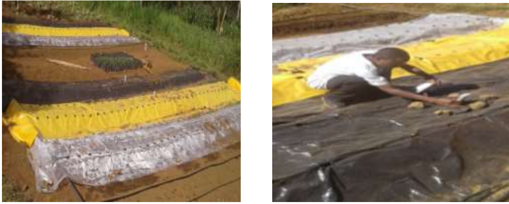
Figure 6: Soil temperature measurement and layout of plastic mulches
