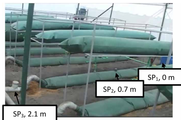
Figure 1 | Plug flow digester layout; digesters on the floor, biogas collection bags directly above; sampling points at different length of the digester are indicated as SP 1 , SP 2 and SP 3 , respectively.
